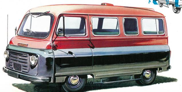
For P.S.V. or hospital and welfare work a raised roof must be included. This is simply achieved on the factory-built P.S.V. Omnicoach and on approved conversions which have to conform to these special regulations.
