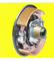
The brake systems on both J2 and J4 vehicles are hydraulically operated, by pendent pedal, on all four wheels. Each system is carefully balanced and compensated to provide maximum braking power under full load. For parking purposes the hand brake operates mechanically on the rear wheels.
