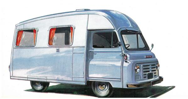
Most of the motor-caravans which are conversions from the factory-built coach or van models have either a fixed raised roof or a lifting roof to provide at least 6 ft. (1.83 m.) of interior head room. While the raised roof allows freedom of movement along the interior, a folding roof does have the extra advantage of lower overall height when on the move or where garage height is restricted.
