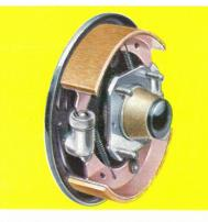
The brake systems on both J2 and J4 vehicles are hydraulically operated, by pendent pedal, on all four wheels. Each system is carefully balanced and compensated to provide maximum braking power under full load. For parking purposes the hand brake operates mechanically on the rear wheels.
