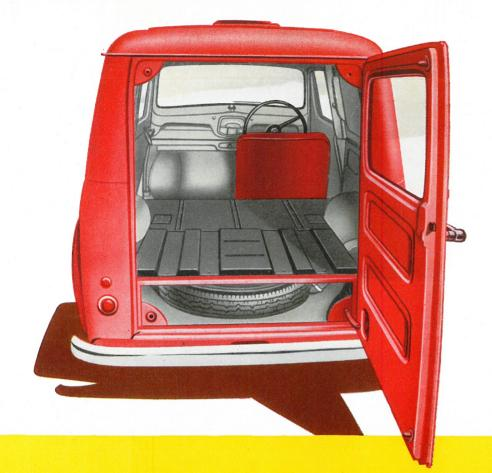
The wide rear door opening affords easy access to the load space. The opening of the door is restricted to prevent it projecting beyond the width of the van.
