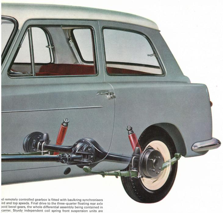
led by hydraulic shock absorbers and an interconnecting stabliising
