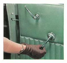
Swivelling louvres are fitted in each door to provide controlled ventilation, and the windows can be quickly raised or lowered by means of the winding handle.
