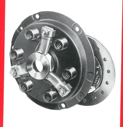
The smooth take-up of power from the O.H.V. engine of the Seven is effected by means of a sturdy Borg and Beck clutch. It is of single dry plate design, having a spring cushion drive and a diameter of  $6\frac{1}{2}$  in. The carbon ring self-lubricating withdrawal bearing is actuated by adjustable linkage. So far as the driver is concerned, the pedal is easy to operate, only very light pressure being required to disengage the mechanism and achieve a silent change of speed.
