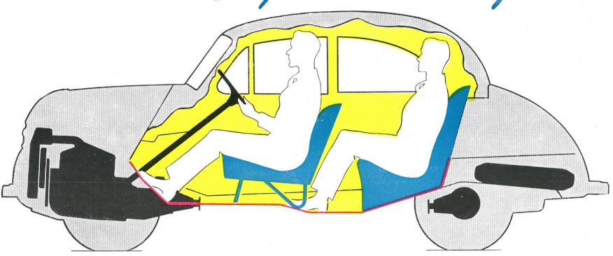
The new Morris Minor was conceived with no concessions to compromise. It is a big car scaled down—but it is a car designed on new principles with traditional skill. By a fundamental change in weight distribution a correct degree of balance has been obtained and unnecessary weight has been saved with an increase in strength.
