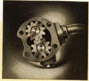
New, larger-capacity oil pump provides pressure lubrication to all engine bearings and other moving parts. Greater oil circulation reduces friction, heat and wear; gives you longer engine life, smoother operation.
