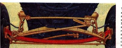
You will be amazed at the remarkable steering ease and stability of the new Ford car. Dual lateral stabilizers, front and rear, reduce sidesway and steady the car on curves or in a crosswind...add to safety, comfort and
