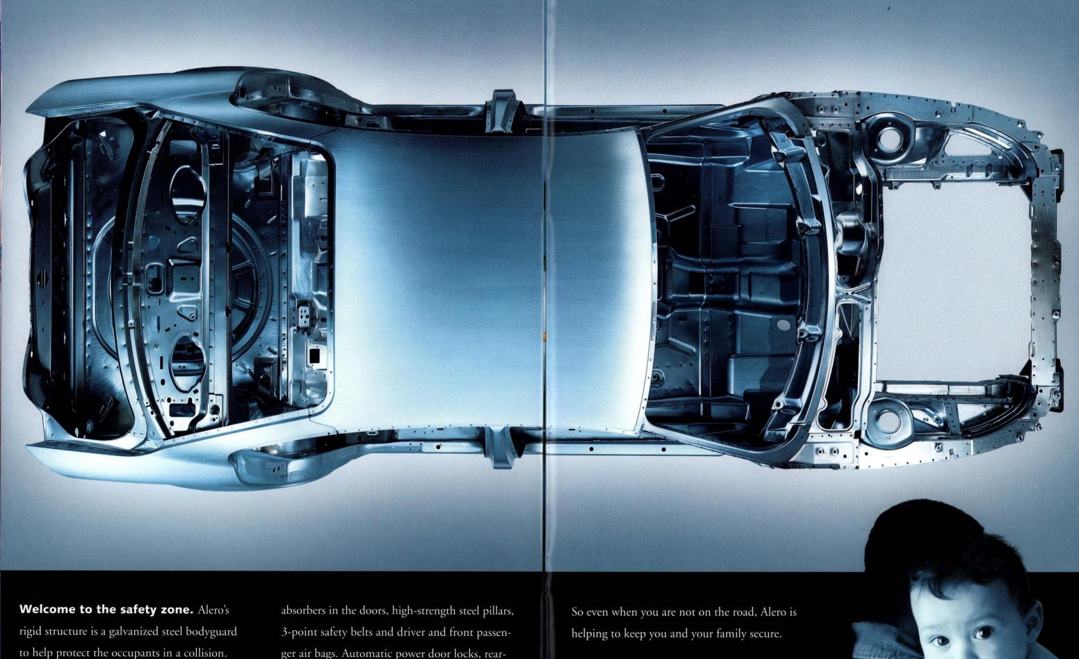
Welcome to the safety zone. Alero's rigid structure is a galvanized steel bodyguard to help protect the occupants in a collision. But that's just the first line of a 'defense system' that goes much deeper. It includes front and rear crush zones, side-door beams, foam energy
