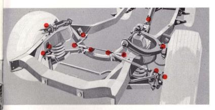
POWER LUBRICATION (MULTI-LUBER)\*—Touch the button on the instrument panel, and your car is completely lubricated at all front suspension and steering system points. You enjoy maximum riding and handling ease all the time.
