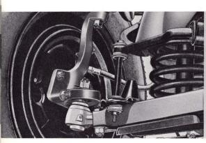
BALL-JOINT FRONT SUSPENSION DESIGN provides great strength and durability, virtually eliminates "bind." Widely spaced ball-and-socket joints increase stability and reduce road shock; require only 4 lubrication points.
