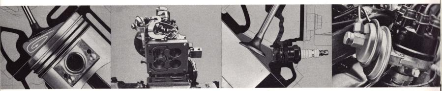
NEW COMBUSTION CHAMBER DESIGN creates greater fuel turbulence for faster, more efficient burning. High-lift valves and larger ports improve intake and exhaust "breathing" for smoother operation.
