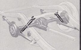
FLAT-ANGLE "SEA-LEG" SHOCK ABSORBERS are teamed with Mercury's long-leaf springs to give you controlled riding comfort, too. Cushions road shock vertically and horizontally. Tension-type spring shackles automatically adjust spring reaction to the car's weight load for easier traveling.
