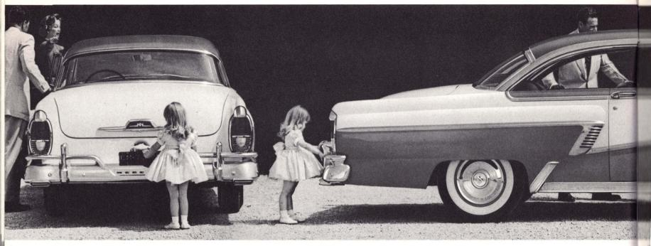
CENTER-FILL GAS TANK located behind the hinged license plate holder lets you drive to either side of pump stand—eliminates scratching of the trunk or fenders by the hose.
