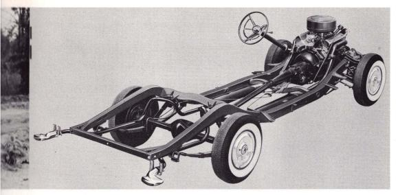
Every Mercury body style has a custom frame designed to its special structural needs. Low engine placement within the frame means better balance of weight, contributing to outstanding roadability.
