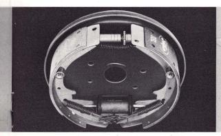
BIG, NEW SAFETY-GRIP BRAKES with more than 190 square inches of braking area provide a new fixed-anchor feature which reduces service points to a single adjustment in each drum. Mercury's power brakes are also improved for still easier and more efficient "power-off" operation.
